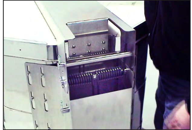
The properly Installed spring-hinge shown closed.
