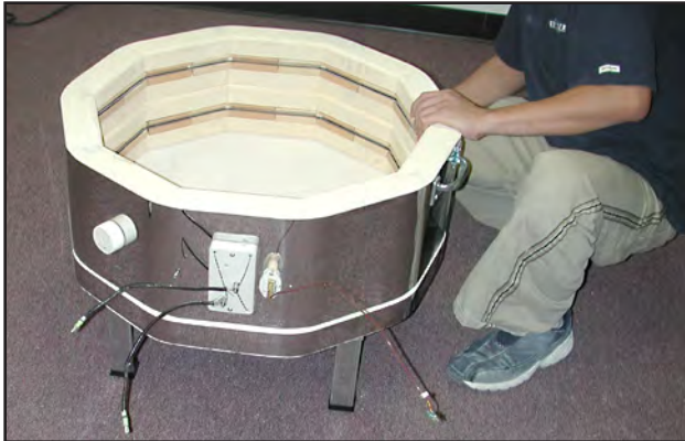
Positioning the bottom ring on the base.
